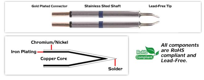
Thermaltronics tip cartridges will typically idle within a temperature range of +/-1.1°C. However, there is variation in idle temperature across tip geometries within an individual temperature series. Thermaltronics offers a wide variety of tip geometries from 0.25mm fine point tip to 5mm chisel. The length and geometry of a tip will have an influence on the tip idle temperature. To accurately measure idle temperature it will depend greatly on the measurement method,
