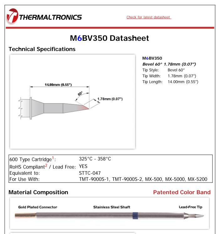
Chromium/Nickel Iron Plating Copper Core Solder All components are RoHS compliant and Lead-Free.
