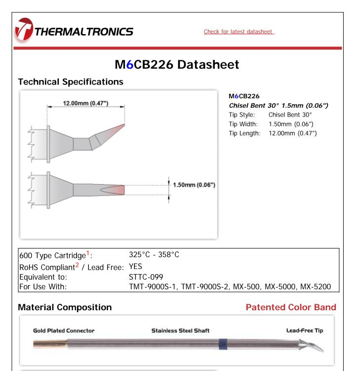
Copper Core Solder 1 Thermaltronics tip cartridges will typically idle within a temperature range of +/-1.1°C. However, there is variation in idle temperature across tip geometry
