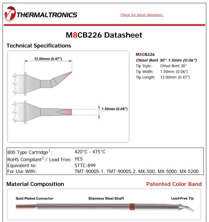
Chromium/Nickel Iron Plating Copper Core Solder
