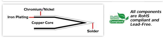
1 Thermaltronics tip cartridges will typically idle within a temperature range of +/-1.1°C. However, there is variation in idle temperature across tip geometries within an individual temperature series. Thermaltronics offers a wide variety of tip geometries from 0.25mm fine point tip to 5mm chisel. The length and geometry of a tip will have an influence on the tip idle temperature. To accurately measure idle temperature it will depend greatly on the measurement method,
