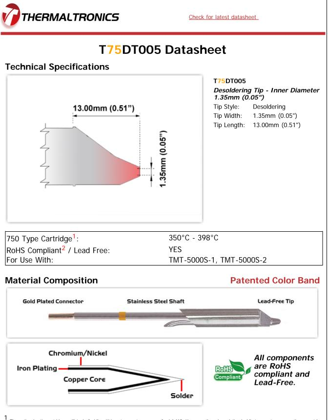
I Thermaltronics tip cartridges will typically idle within a temperature range of +/-1.1°C. However, there is variation in idle temperature across tip geometries within an individual temperature series. Thermaltronics offers a wide variety of tip geometries from 0.25mm fine point tip to 5mm chisel. The length and geometry of a tip will have an influence on the tip idle temperature. To accurately measure idle temperature it will depend greatly on the measurement method,
